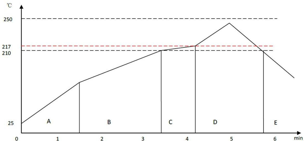
Zone A: Preheat: This raises the temperature at a controlled rate, typically 0.5 - 2C/s. This will preheat the component to 120°C to 150°C to distribute the heat uniformly to the PCB.
